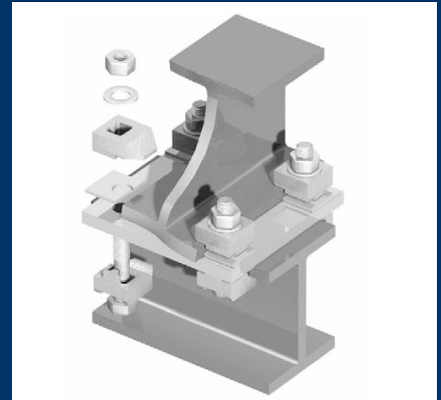
5.9 Suspended beam to beam connections by Lindapter
