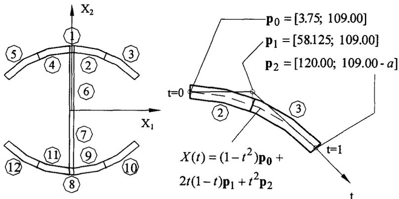
Fig. 5. Cross-section of exemplary beam
