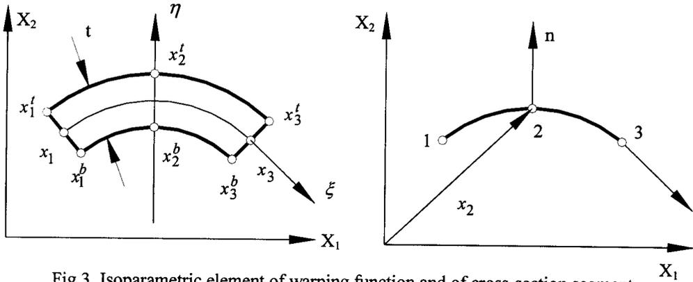
Fig.3. Isoparametric element of warping function and of cross-section segment
