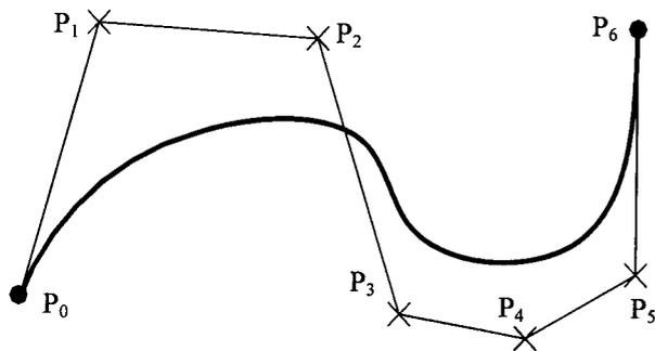
Fig. 2. Examples of Bezier parametrization
