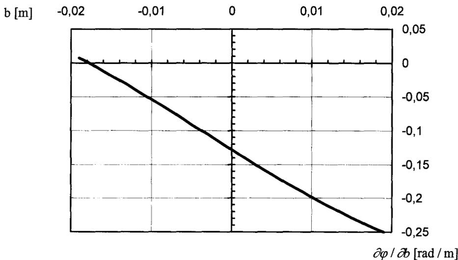
Fig.6. Sensitivity of torsion angle of the beam to imperfection  $b$  of shape of its cross-section
